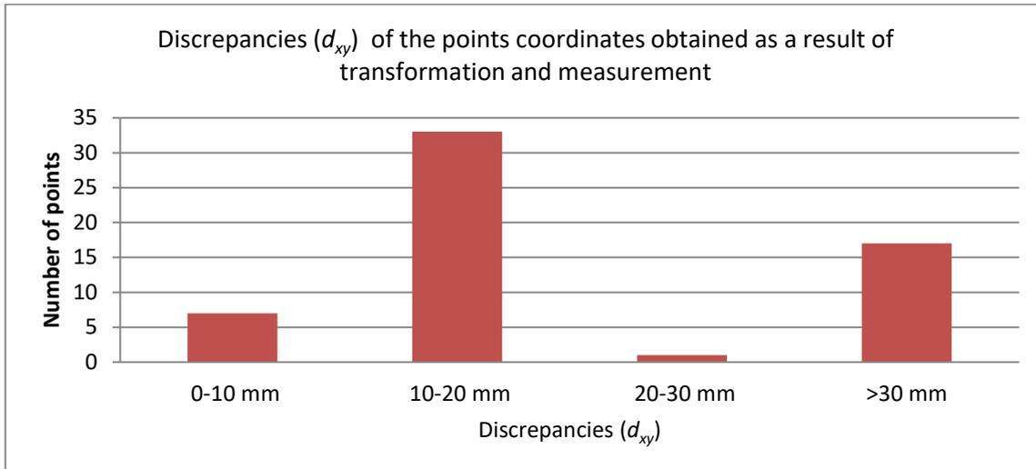
**Figure 4.** Distribution of discrepancies of the coordinates of measured and calculated points as a result of transformation
