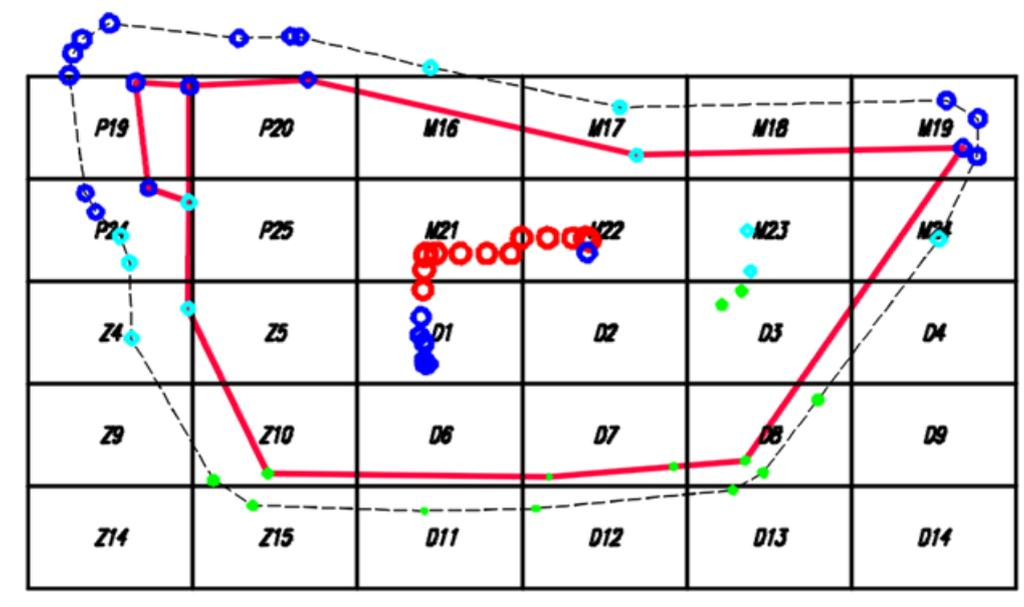
**Figure 3.** Ellipse of the discrepancies of the coordinates of the points in the second-degree conformal transformation between the Borowa Góra and PL – 2000 systems, (description in the text).
