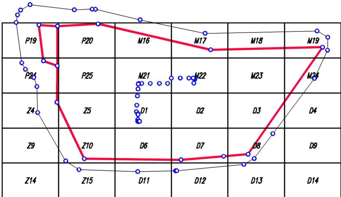
**Figure 2.** Selected joint points constituting the basis of the transformation algorithm between the Borowa Góra and PL-2000 systems.
