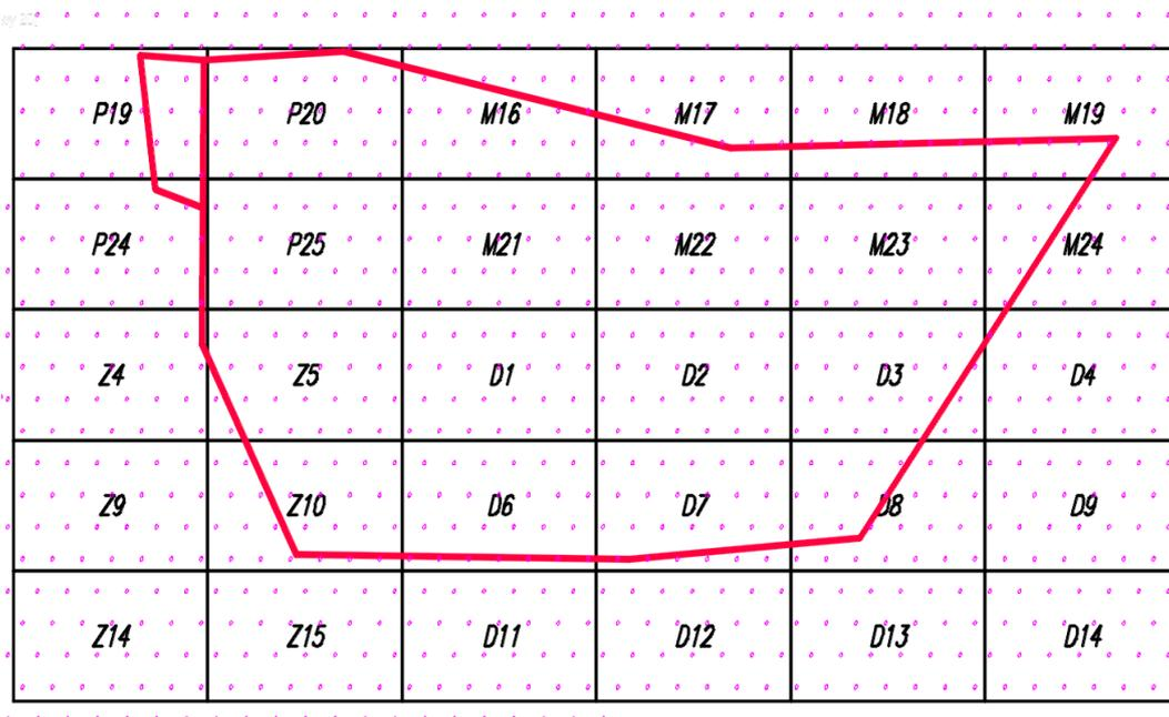
**Figure 1.** Coverage of the mining area of PG Silesia with a grid of test points (250m x 250m) used to pre-determine the optimal type and grade of the transforming polynomial.
